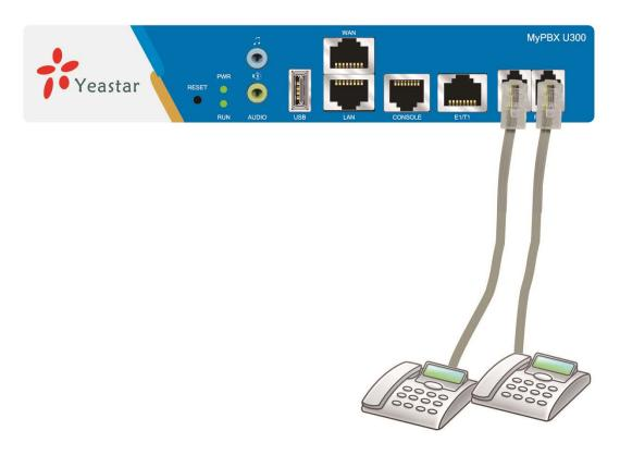
Figure 3-3 Connection of FXS ports
