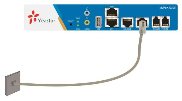
Figure 3-2 Connection of E1/T1 port
