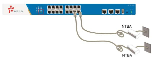
Figure 3-4 Connection of BRI ports and Status LED
