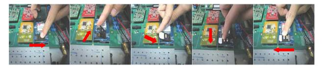
Figure 3-2 Inserting the SIM Card
