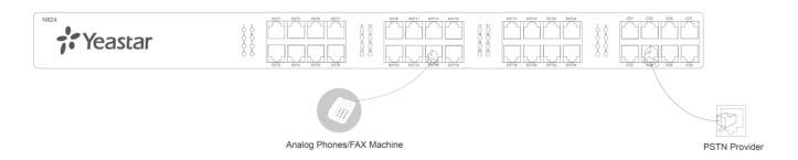
Figure 2-1 N824 Front Panel Connection Diagram
