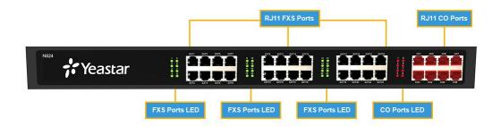
Figure 1-1 N824 Front Panel
