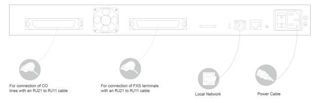
Figure 2-2 N824 Rear Panel Connection Diagram
