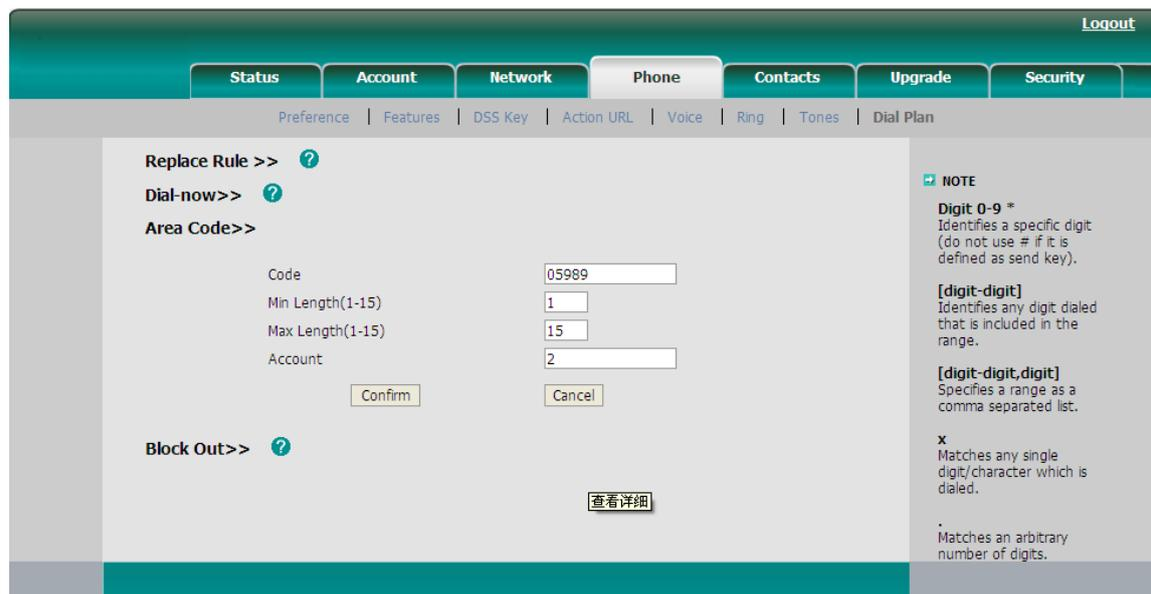
The screenshot shows a web interface for configuring phone settings. The top navigation bar includes tabs for Status, Account, Network, Phone (selected), Contacts, Upgrade, and Security. Below the navigation bar, there are sub-tabs for Preference, Features, DSS Key, Action URL, Voice, Ring, Tones, and Dial Plan. The main content area is titled 'Area Code>>' and contains the following fields:
