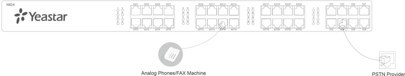
Figure 2-1 N824 Front Panel Connection Diagram
